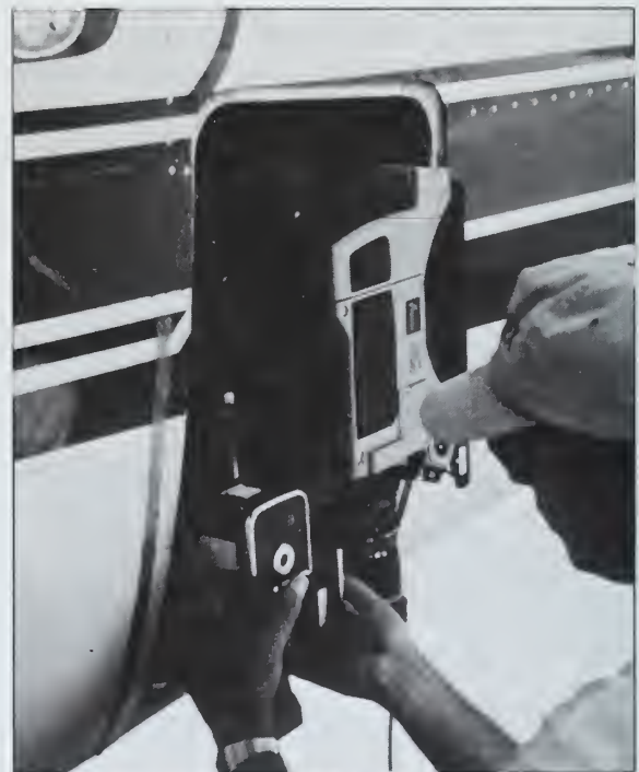
Figure 15. An aerial video camera mounted on a Bell 206 Jet Ranger helicopter and mounted in the luggage compartment of a Cessna 182 light aircraft. Photographs provided by the USFS.
